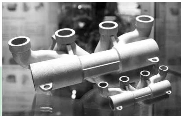
Metal parts produced with a 3D printer – a new challenge in the fight against proliferation
